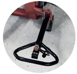
The handle can turn to the side to enable easy operator access
